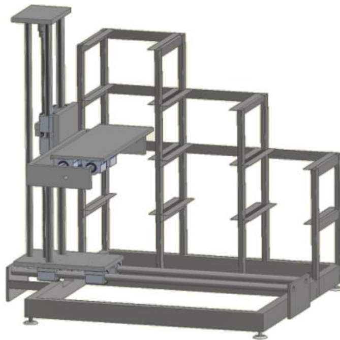
Fig. 8. Main structure of the ASRS machine
