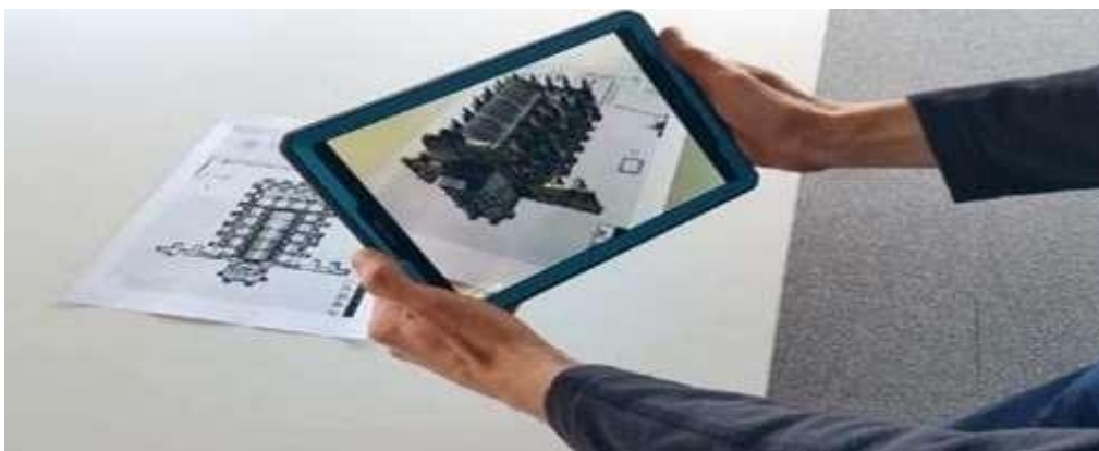
Fig. 27. Augmented reality application overlaying a 3D model of Rosslyn Chapel on top of a tracked 2D target
