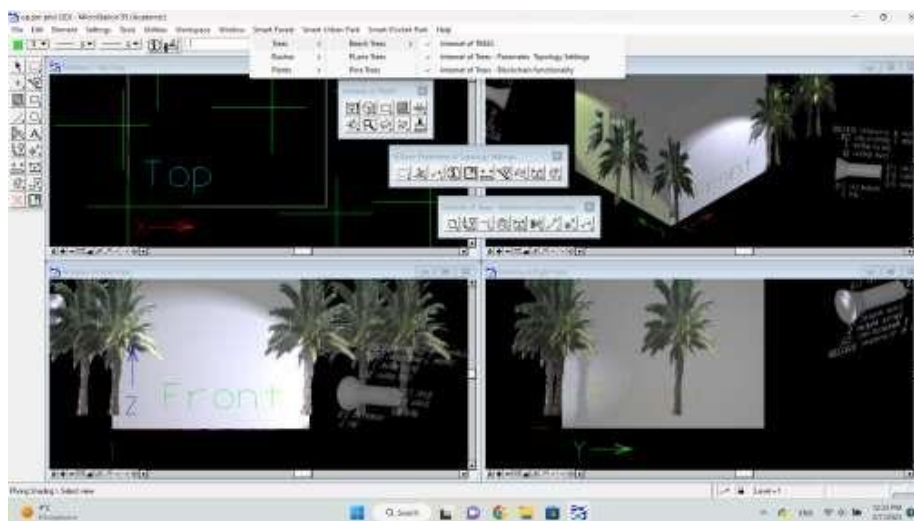
Fig. 23. The three palettes (smart-forest > trees > beech trees): Internet of trees (10 basic CAD tools); Internet of trees – parameter topology settings (10 parametric CAD tools); Internet of trees – blockchain functionality (9 database-CAD connection tools)
