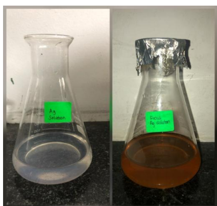
Fig. 2. Colour change exhibited by the prepared F. benghalensis assisted silver nanoparticles
