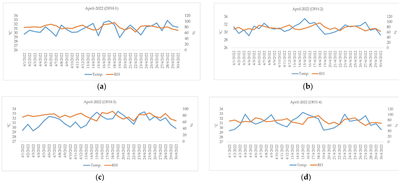
Figure 16. Air temperature ( ^{\circ}\text{C} ) and RH (%) measured from LCSs during the period from 1 to 30 April 2022: (a) DFH-1, (b) DFH-2, (c) DFH-3, and (d) DFH-4.
