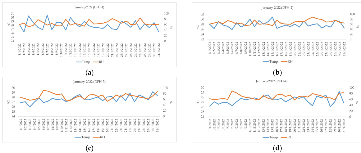
Figure 13. Air temperature (°C) and RH (%) measured from LCSs during the period from 1 to 31 January 2022: (a) DFH-1, (b) DFH-2, (c) DFH-3, and (d) DFH-4.
