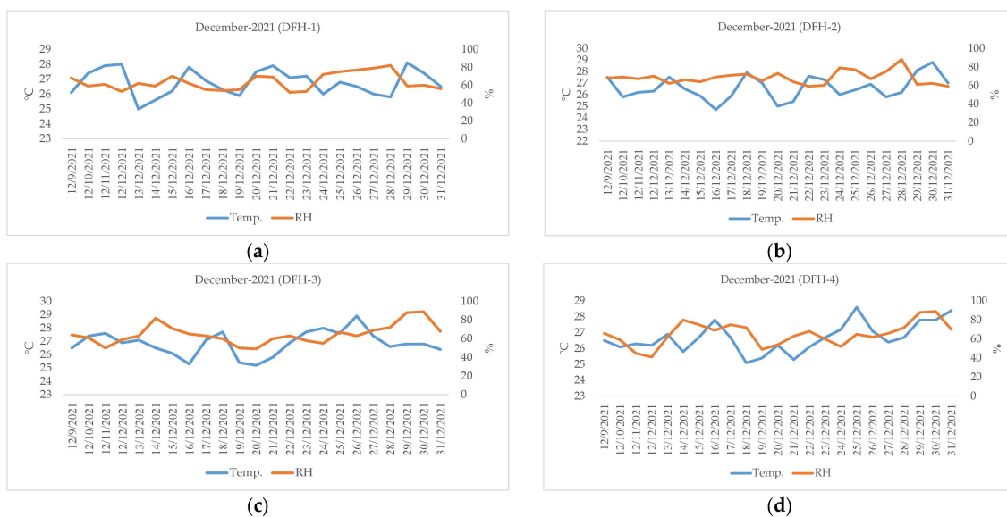
Figure 12. Air temperature (°C) and RH (%) measured from LCSs during the period from 9 to 31 December 2021: (a) DFH-1, (b) DFH-2, (c) DFH-3, and (d) DFH-4.
