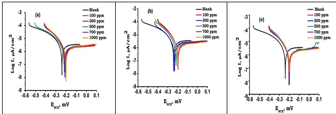
**Figure 1:** Tafel curves for blank and immersed 316L Stainless steel in various concentrations of casein's solutions for: (a) 60 (b) 90 and (c) 120 minutes, respectively.
