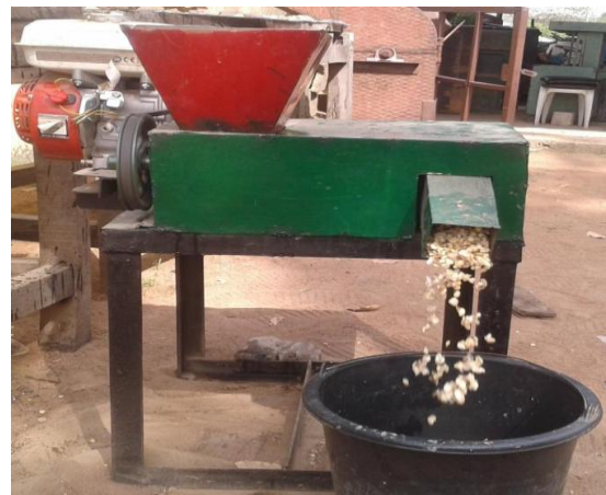
Fig. 5. Cowpea decorticator in operation
