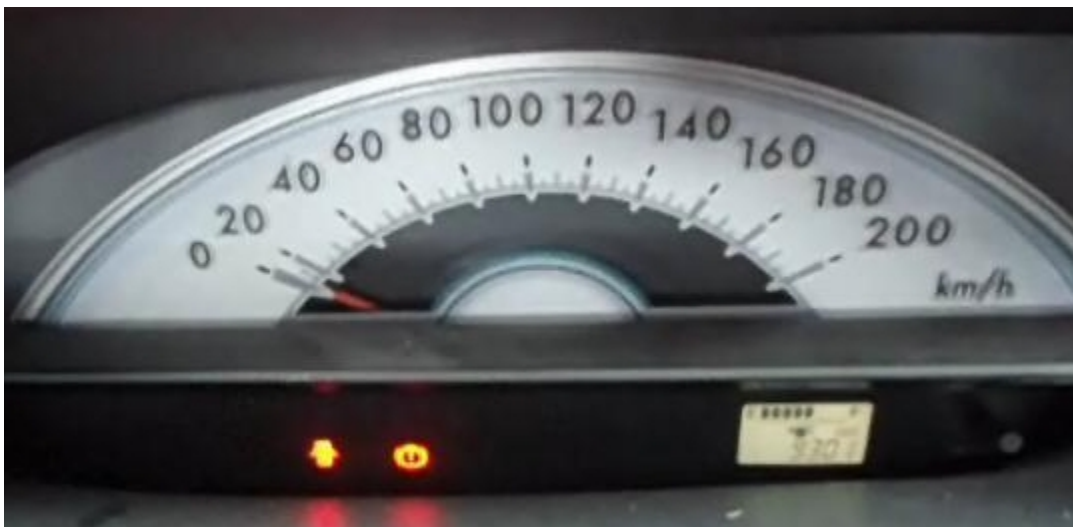
Fig. 9. MIL is off as fault code is cleared.
