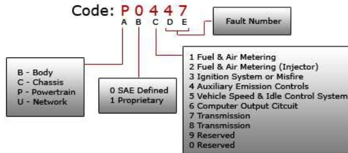
Fig. 2. Format of diagnostics trouble code
