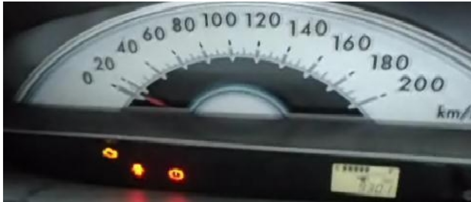
Fig. 6. MIL is ON as fault is created.
