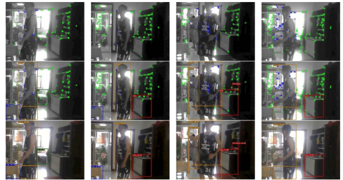
Figure 6. Experiment with a monocular camera in a real-life scene. Our method successfully detects dynamic points belonging to known objects (people) and limited unknown moving objects (plastic bags).
