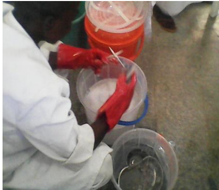
Fig. 5. Washing instrument wearing Non-disposable water-proof Gloves in soap solution after soaking in Hexanious solution for 15 min
