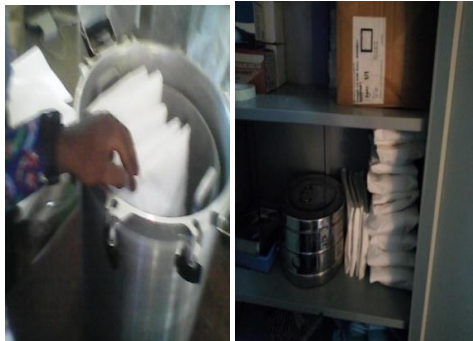
Fig. 11. Proper loading of the autoclave pot/ storage of sterile packs in cabinet
