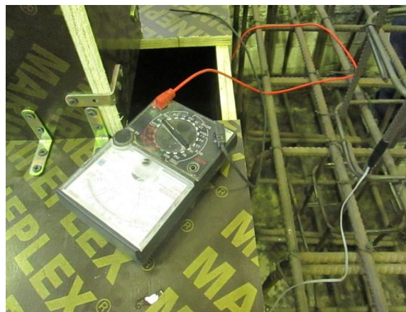
Fig. 3. Calibration of the strain gauges
