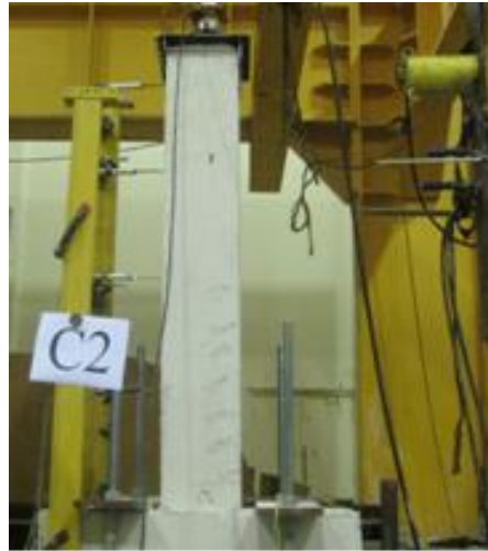
Fig. 6. The cracks of C2 column under the lateral loads
