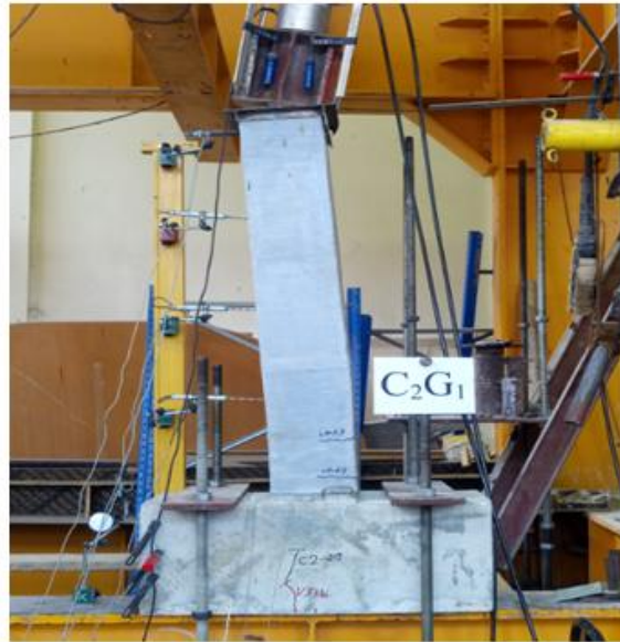
Fig. 9. The cracks of column C2G1 at failure under the ultimate axial load
