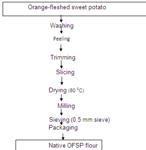
Fig. 1. Flow chart for the production of native orange-fleshed sweet potato (OFSP) flour
